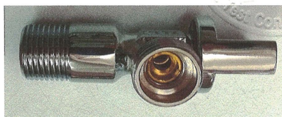
Figure 3 - Surface of internal water passage
