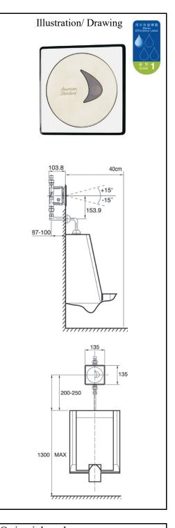
Note: WF-8014.0S0.50= WF-8004.0S0.50 (WSD approved ) + AC circuit board
