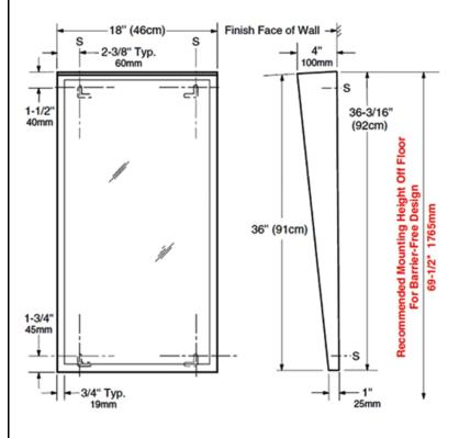
Frame — 18-8 S, type 304, heavy-gauge stainless steel with satin finish. Tapers from 4" (100mm) depth at top to 1" (25mm) depth at bottom. Bevel design on front holds frame tightly against mirror. Corners are welded, ground, and polished smooth. Galvanized steel back and inner stiffener frame is one-piece welded construction with slots for mounting screws and integral screw-head lock.
