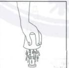
7. IMPORTANT: SAND AND RUST MOVE THROUGH WATER PIPES. ALWAYS CLEAR DEBRIS FROM WATER LINE TO COMPLETE INSTALLATION: Remove TOP ASSEMBLY with a 1/8 turn counterclockwise. While holding a container over the uncapped VALVE to prevent splashing, turn water supply on and off a few times. Replace TOP ASSEMBLY by engaging lugs and rotating 1/8 turn clockwise.
