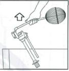
2. Flush tank and sponge out remaining water. Remove old ballcock assembly.
