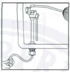
1. Shut off water supply to tank
