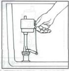
8. Turn on water supply. Adjust water to desired level by squeezing WATER LEVEL ADJUSTMENT CLIP and moving FLOAT CUP up or down along stainless steel link
