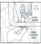
4. Push down on the VALVE SHANK (not the TOP) while tightening LOCK NUT. Hand tighten only. DO NOT OVERTIGHTEN or tank may crack. Make sure FLOAT CUP does not touch toilet tank walls, trip mechanism or flush valve
