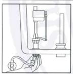
5. Tighten water supply connector. Hand tighten only. DO NOT OVERTIGHTEN or tank may crack.
