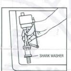
3. Place SHANK WASHER on threaded shank of new VALVE. Position valve in tank
