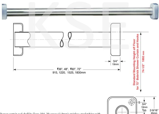
Shower curtain rod shall be Type-304, 20-gauge (1.0mm) stainless steel tubing with satin finish and 1" (25mm) outside diam-eter. Flanges shall be Type-304, 20-gauge (1.0mm) stainless steel with satin finish and drawn, one-piece, seamless onstruction.
