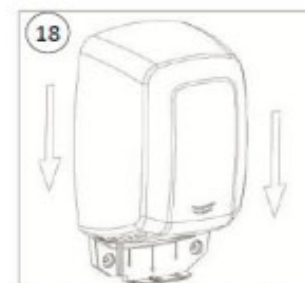
Mount the dryer over the Plug-in base with a from top to down movement
