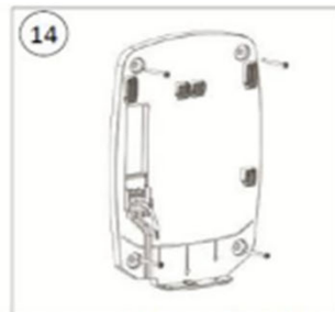
Screw the Plug-in base to the wall(x4)
