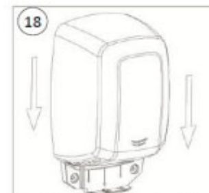
Mount the dryer over the Plug-in base with a from top to down movement
