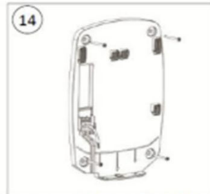
Screw the Plug-in base to the wall(x4)
