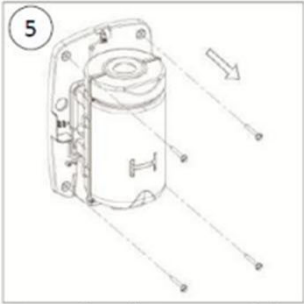
Unscrew the wall mount screws (x4)
