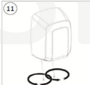
Screw the cover fixing screws (x2) Your dryer is now ready to be used on a Plug-in base
