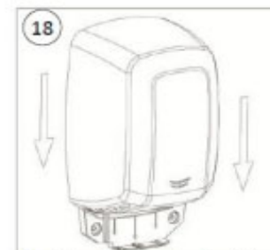
Mount the dryer over the Plug-in base with a front to back movement
