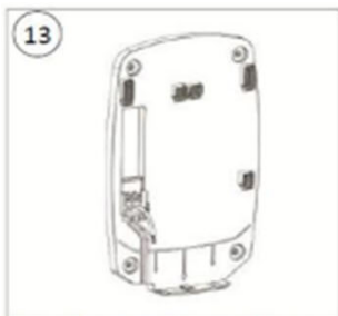
Route the wires through the Plug-in base as shown on the picture
