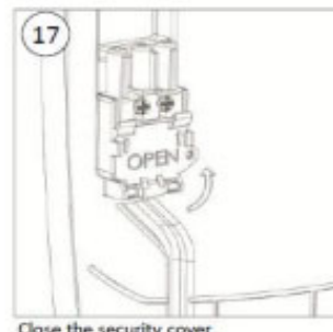
Close the security cover Your Plug-in base is now ready to be used with a Plug-in dryer
